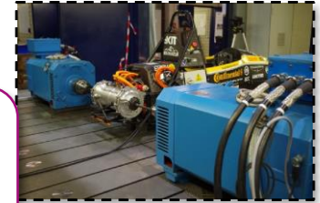
X-in-the-Loop Test Deployment View
